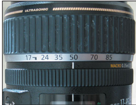
FIGURE 7.46 This 17–85 mm lens is currently set to a focal length of 50 mm. However, this lens is attached to a Canon EOS SLR that has a focal length multiple of 1.6. Therefore, the crop of this lens is equivalent to 50 \times 1.6 , or 80 mm. Our minimum shutter speed for sharp handheld shooting is 1/80^{\text{th}} of a second. However, because the lens has a 3-stop image stabilizing system, we might be able to get away with shooting as low as 1/20^{\text{th}} .
